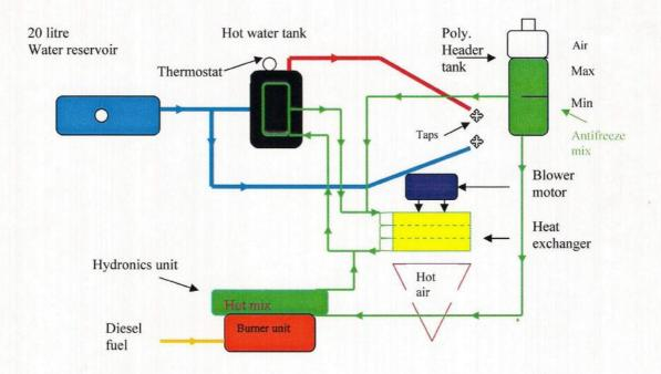
The Hydronic burner unit is fitted under the vehicle and is fuelled from the vehicles Diesel system. A mixture of water and antifreeze passes through the system and transmits its heat to the water tank and hot air system.
