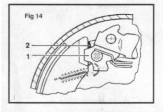
Transmission lever (1) must abut the adjuster housing stop (2).
