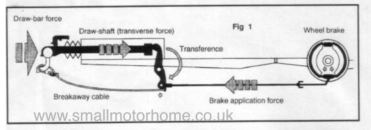
The overrun device can be described as the control device of the overrun brake system. A draw-bar force is produced at the coupling point by reducing the speed of the towing vehicle. After the threshold level has been passed, the draw shaft is pushed in, thus actuating the overrun lever, the wheel brakes (1 & 2) are then applied via the expanding clutch (3) (Fig 2)
